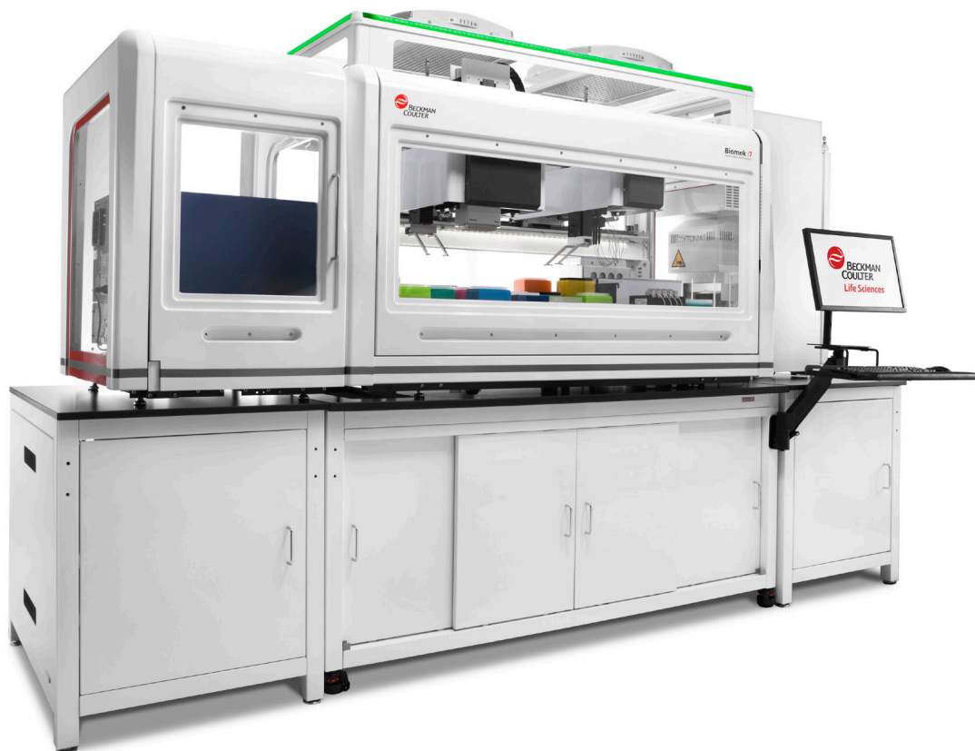
Figure 3. The Biomek i7 Workstation, along with various integrated devices, was used to automate a cell line development workflow.
