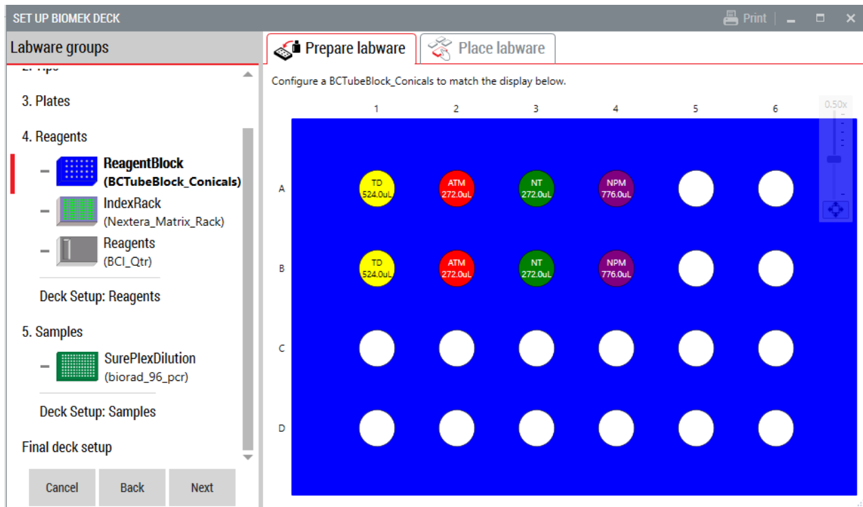
Figure 5A. Guided Labware Setup indicates reagent volumes and guides the user for correct deck setup
