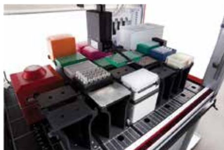
Figure 1. Biomek i5 Span-8 Genomics Workstation with optional enclosure on a Biomek Cart. High Capacity deck layout for increased walk away time.
