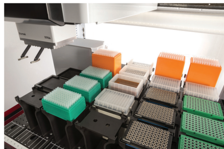
Figure 1. Biomek i5 Multichannel 96 Genomics Workstation with optional enclosure on a Biomek Cart. Large Deck capacity to increase walk away time.
