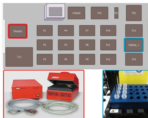
Figure 2. Biomek FX P deck configuration (top). Biometra TRobot (bottom left) offers fully automated enzymatic incubations and thermocycling while the Static Peltier unit (bottom right) provides chilled enzyme master mix storage during the course of the run.
