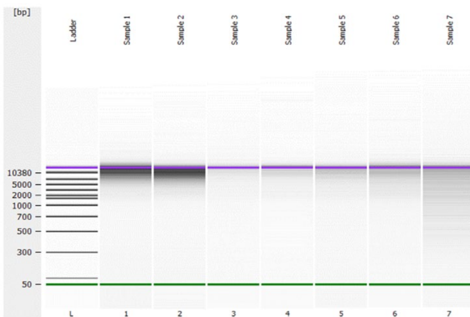
Figure 6. Extracted DNA was analysed with Agilent Bioanalyzer 2100 with Agilent DNA 12000 kit and DNA chip.
