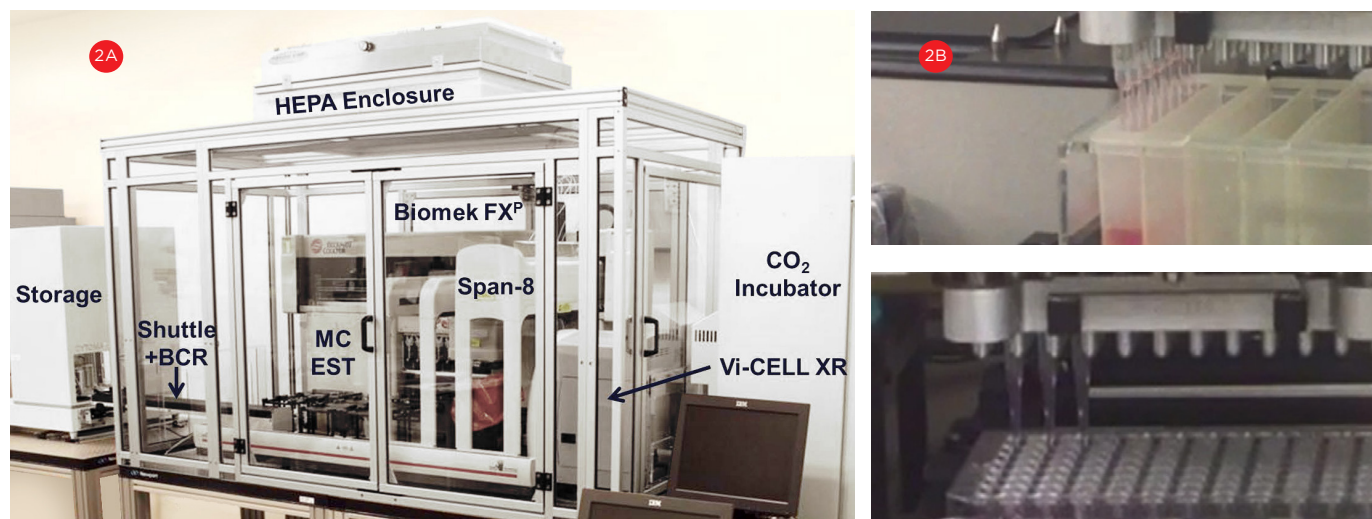
Figure 2. Cell culture system. A) A Biomek FX P Workstation with a 96-channel head and Span-8 pipettors inside a HEPA-filtered enclosure for automating sterile cell manipulations. 3D cultures were grown in HDPs in an integrated incubator for complete workflow automation. B) The 96-channel head utilized enhanced selective tip pipetting which provides additional flexibility by enabling any pattern of tips to be used.
