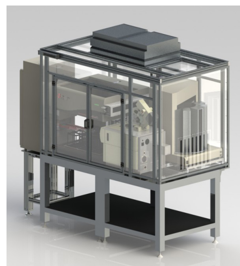
Figure 8. Automated HDP Compound Screen. A rendering of a potential HDP screening system that utilizes imaging as the primary assay. Plating, treatment, and staining could be completed using a Biomek NX P Workstation with a 96-channel EST head while analysis is performed on an integrated ImageXpress Micro.
