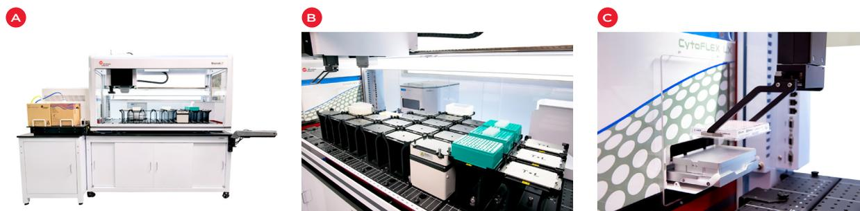
**Figure 1.** **A)** \*Biomek i7 Multichannel workstation with Integrated CytoFLEX LX Flow Cytometer. **B)** Biomek i7 Multichannel workstation deck with the integrated CytoFLEX LX flow cytometer. **C)** An enhanced view of automated loading of a 96-well plate into the CytoFLEX LX flow cytometer with the Biomek gripper.
