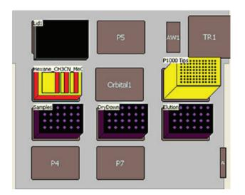
**Figure 2.** Deck layout on the Biomek NX<sup>p</sup> Workstation configured for preparation of serum samples, prior to the analysis of 25-OH-VitaminD2 and D3 by LC/MS/MS.
