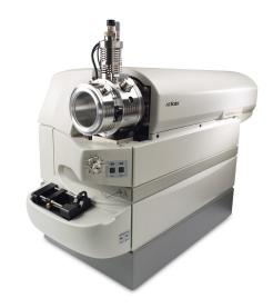
Figure 1B. AB SCIEX 3200™ QTRAP® LC/MS/MS System.
