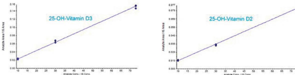
**Figure 6.** Calibration curves for 25-OH-Vitamin D3 and D2, with manual sample preparation.
