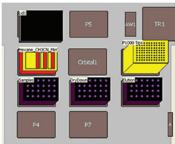
Figure 2. Deck layout on the Biomek NX<sup>P</sup> Workstation configured for preparation of serum samples, prior to the analysis of 25-OH-Vitamin D<sub>2</sub> and D<sub>3</sub> by LC/MS/MS.
