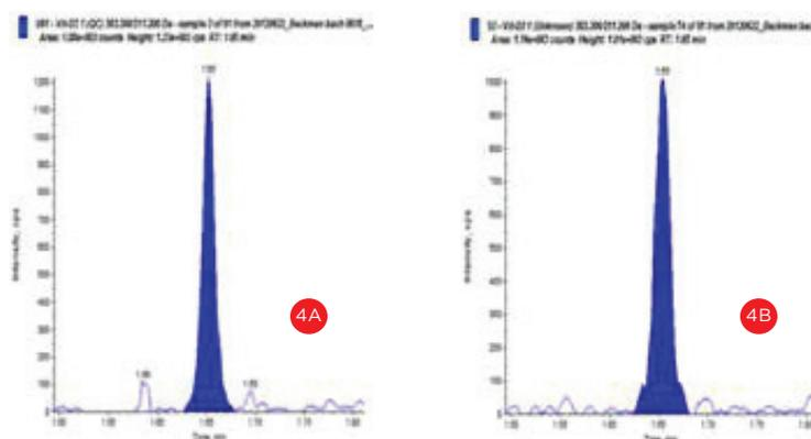
**Figure 4A and 4B.** Representative chromatograms for serum standards containing 10 ng/mL of 25-OH-Vitamin D3. A: Automated sample preparation using Biomek NX<sup>P</sup> Workstation. B: Manual sample preparation.
