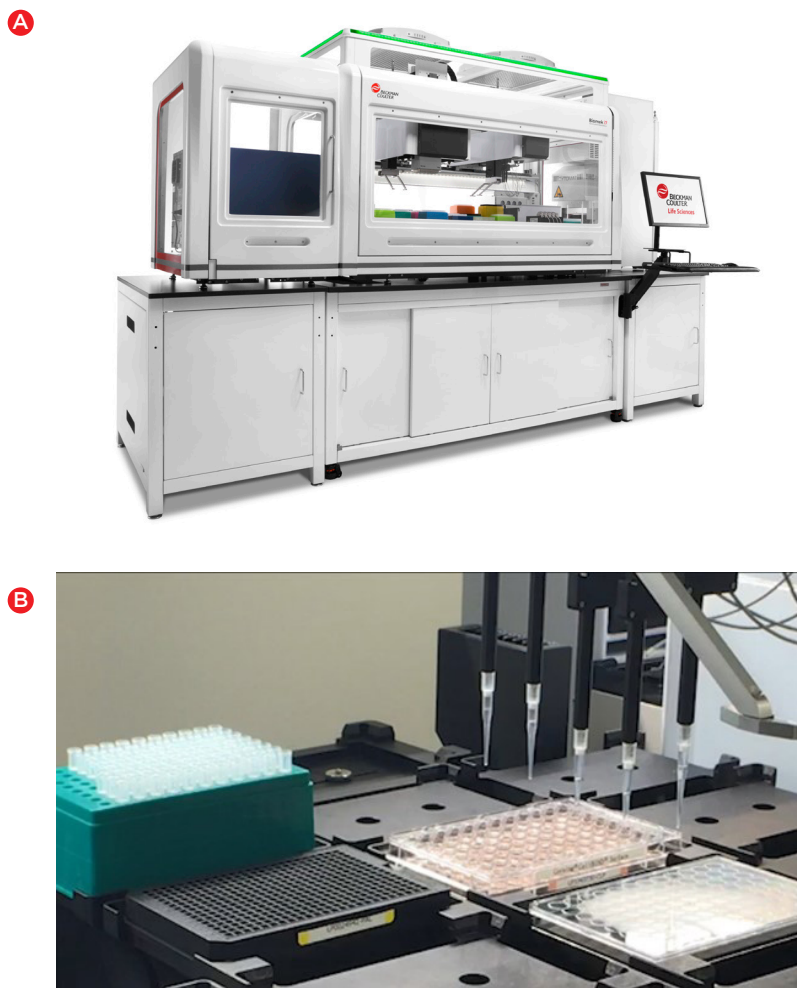
Figure 2. Automated hit picking. A) Biomek i7 with HEPA filters and integrated devices utilized for cell line development. B) Media from the ~15% of wells with colony growth from a single cell were sampled using the Span-8 pipettors and transferred to a black 384-well Tilted Well Plate for analysis on the Octet HTX (Pall Forte Bio).
