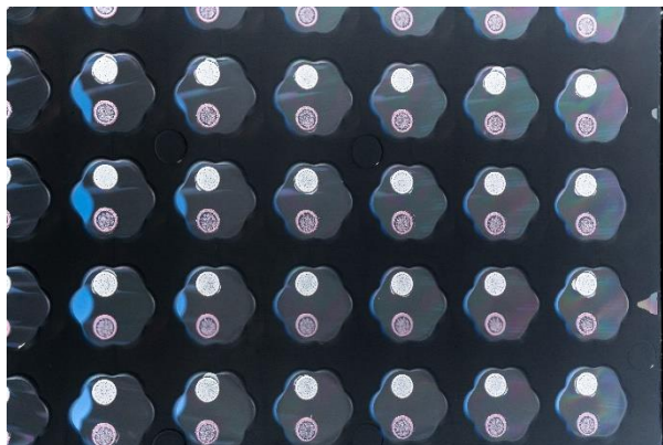
Figure 4: Bottom of the MTP, displaying measurement sensors for pH (white) and DO (red)
