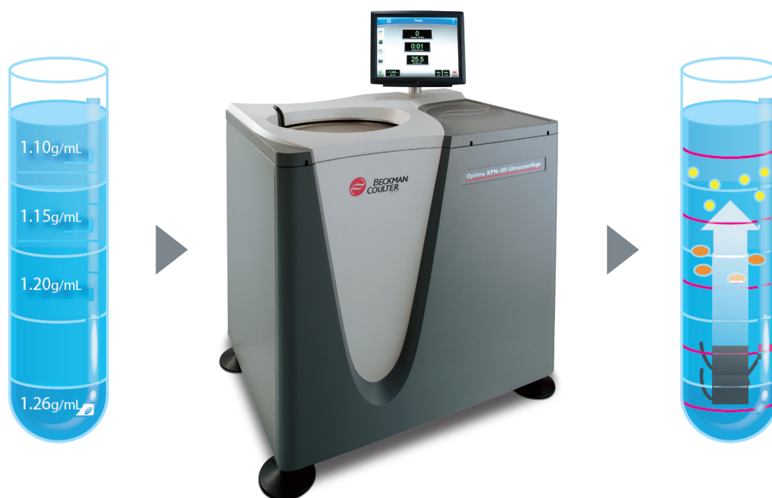
Figure 4. Isolating EVs involves the removal of contaminants and the separation of EVs from other particles, such as chylomicrons and lipids, present in biological fluids or cell culture media. Ultracentrifugation utilizes centrifugal force to separate components based on their size and/or density. Differential ultracentrifugation techniques employ multiple spins at progressively increasing speeds to first eliminate contaminants and then pellet EVs. Density gradient ultracentrifugation is a high-resolution purification technique that relies on a medium with graded densities, such as sucrose or iodixanol, to separate particles based on their physical properties such as size, shape, mass, and density.
