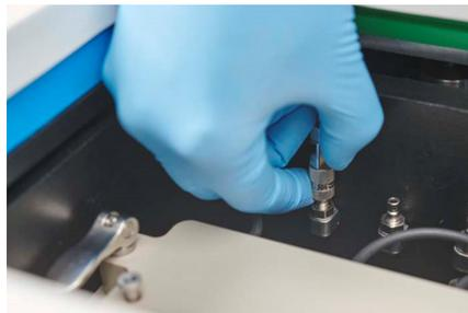
**Figure 15.** Removing the gassing lid out of the incubation chamber.
