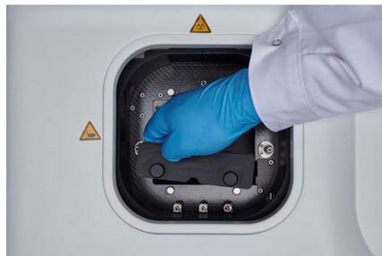
**Figure 12.** Placing the adapter plate into the 32-mode position.
