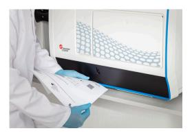
Transfer target values from the assay sheet with the barcode scanner
